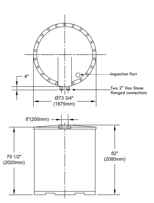
**NOTE:** Tolerance for all dimensions is  $\pm 1/2$ " (12.5 mm)
